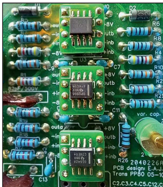
Photo 3: Here, the SOIC8-DIP8 adaptors have been added to enable easy op-amp exchange or repair.
