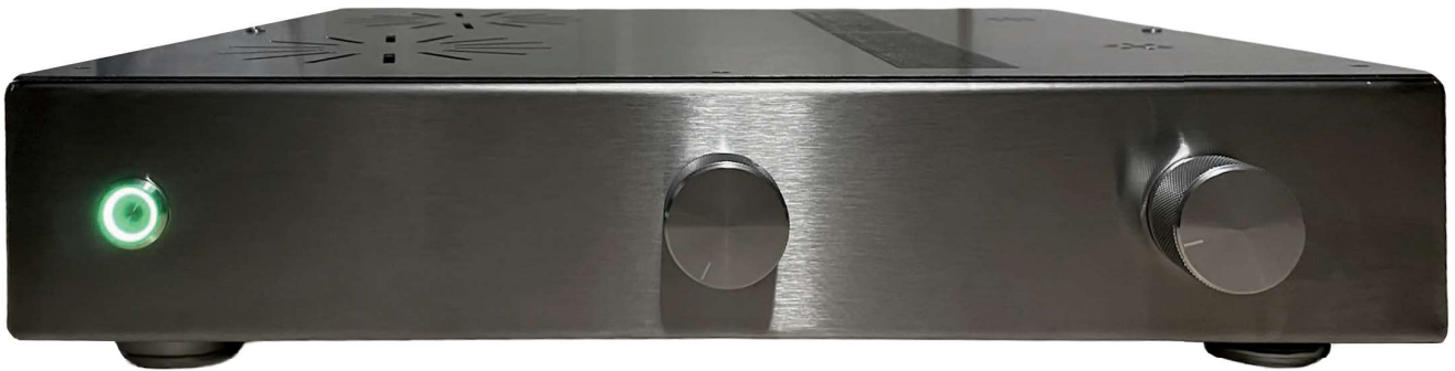
Photo 1: This is the finished version of the TubeSociety 2022 OTL Hybrid Tube Amplifier, a non-feedback hybrid design with a tube driver and a push-pull MOSFET output section.
