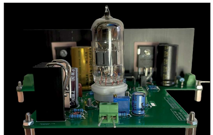
Photo 2: This amplifier, built by Erwin Reins, paralleled the two triodes inside one ECC88 tube for smallest effective plate resistance and optimal linearity.
